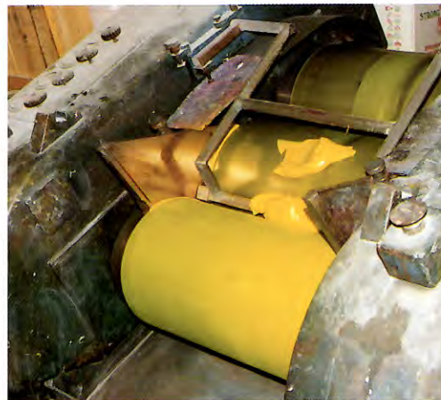
In oil paint production, machine-operated mills are used by paint manufacturers to grind large quantities of pigment into oil to make paint.
