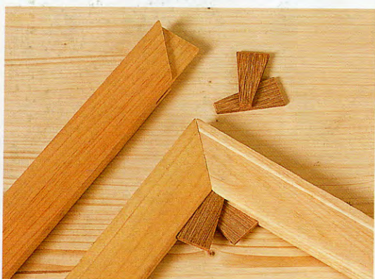
Slotted expandable lap joint with wedges
